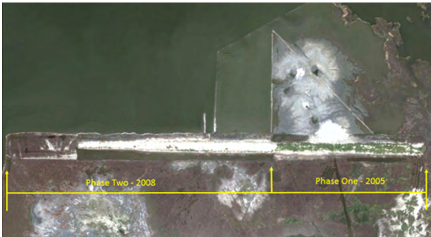
Port Fourchon created a man-made ridge using dredge material. Image: Port Fourchon
